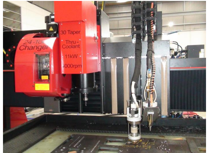
K3000xmc Machine Showing from RHS: 24 Automatic Toolchanger 11kW Spindle two spare vertical stations Hypertherm HPR400 Plasma Oxy Fuel torch
