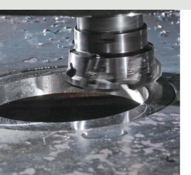
Whether you're drilling or tapping, no matter which machine you choose you're bound to need a slightly bigger hole. So why limit yourself to a maximum hole size? If your machine includes hole interpolation and thread milling capabilities, you'll be able to create perfect threaded holes of any size. When you're not limited by the types and sizes of holes you can produce, you can take on more jobs, process more plate, and boost your bottom line.
